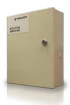
The FP1135 Isolation Amplifier connects to an existing 100V speaker line and reproduces this signal at up to 60W load on a separate supervised 100V line. It is suitable for use with speech, music and warning tones. The 100V output line from the amplifier is electrically isolated from the input 100V line, thus separating noise or other signals on the input line from the output. The Isolation Amplifier requires a nominal supply of 27Vdc.
