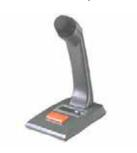
The SU0169 Paging microphone is a desktop dynamic microphone with a cardioid polar pattern. It features a short-off press to talk switch with an open-off type extra switch. It has low handling noise and a 600 ohm balanced output impedance. The SU0169 is finished in a grey ABS body with a zinc plated wire mesh head. Compatible with FP0539 and FP0902 Paging Consoles.
