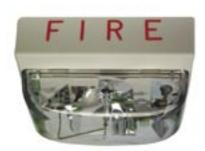
The 4906-9104 Multi-Candela strobe is a high output xenon strobe capable of signalling evacuation using the ISO 8201 "T3" temporal pattern, as required by AS1670.4-2004 and AS 1670.1-2004. It is ceiling mounted and produces white light with a link-selectable intensity of 15cd, 30cd, 75cd or 110cd. It is usually controlled by the ISO 8201 Strobe Driver Module (PA1043) or a QE90 STRM Strobe Relay Module. A 24V output cannot be used.
