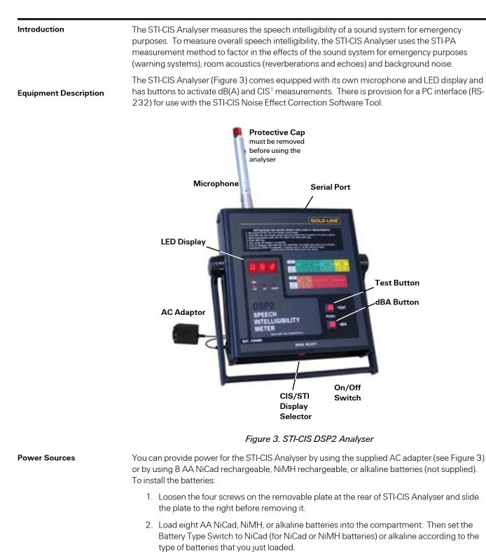
3. Replace plate and tighten down the four screws previously loosened. DO NOT OVERTIGHTEN SCREWS.
