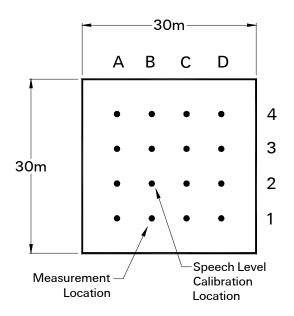
Figure 14. Example Test Locations
