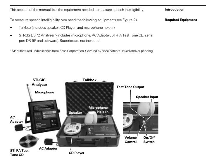
Figure 2. Equipment required to Measure Speech Intelligibility
