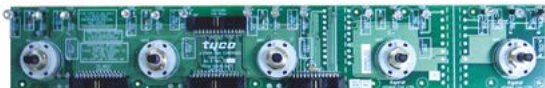
KT0478 Kit, AS 1668 5 way Fan Control Module (Includes PCB, 5x switch knobs and caps, 5x panel labels, 2x 26W FRC 2m cables, LT0368 instructions). Optimised for use with MX4428 IOR.
