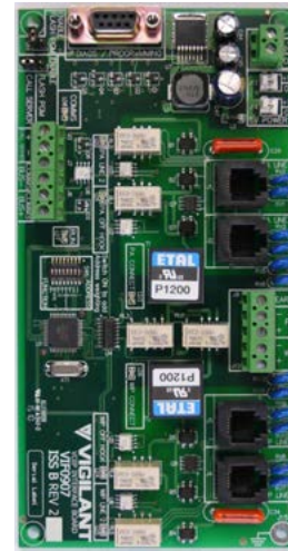
PA0644 VIF0907 VoIP Interface incl. 1x LM0448, 2x LM0552, DIN rail mntg h'ware
