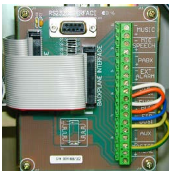
PA0657 SE9004 Signal Interface
