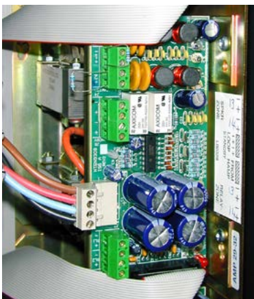
PA0691 HTRN9308-1 2x50W Transformer Module
