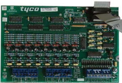
FP0553 , F3200 8 Zone Input Expansion Kit Includes: PA0492, 8 Zone Module, LM0053 FRC, 8 x EOLR (std). (EOL = 2k7 5% 0.4W). Size: 195 x 125 x 12mm, 220g
