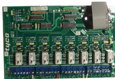
FP0554 , F3200 8 Relay Expansion Kit Includes: PA0493 8 Relay Module, LM0053 FRC, 8 x Minijump links (for supervision selection). Size: 195 x 125 x 12mm 250g
