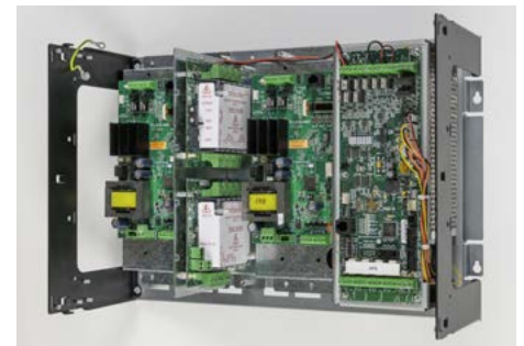
T-GEN 60 on FP1119 Bracket in PDI Expansion Bay with FP1118 Brackets & Splitter Modules
