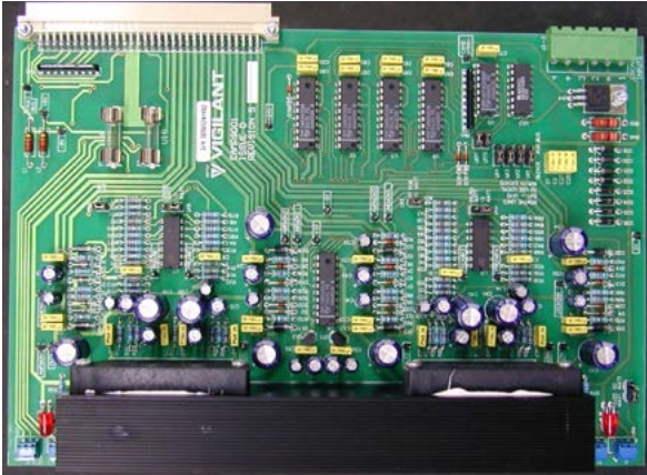
PA0650 EAMP9001 4x10W / 2x25W Zone Power Amplifier PCB Dimensions 233x159x48mm
