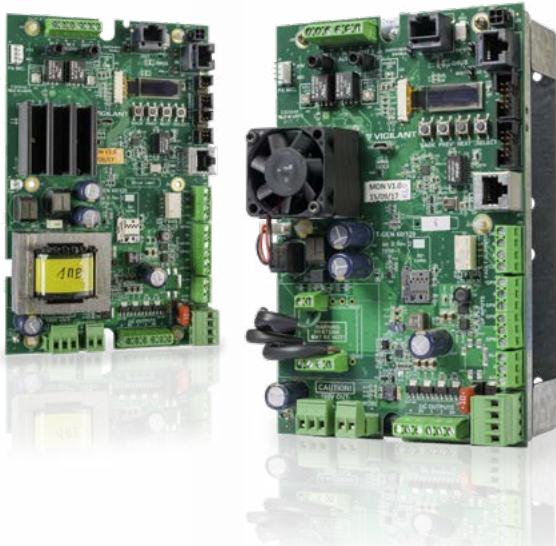
FP1115 T-Gen60 60W Amplifier Module FP1116 T-Gen120 120W Amplifier Module (with fan)
