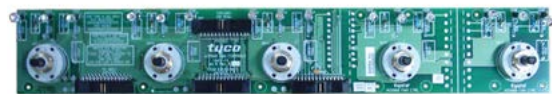
KTO478 Kit, AS 1668 5 way Fan Control Module Includes PCB, 5x switch knobs and caps, 5x panel labels, 2x 26W FRC 2m cables, LTO368 instructions
