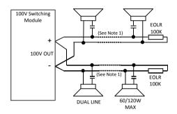
1. Capacitor 10V bipolar. Value 1-5uF per watt of speaker load.
