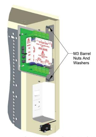
Figure 4 – 100V Switching Module in Slimline MX1 Cabinet
