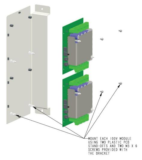
Figure 2 – Two 100V Switching Modules mounting on bracket
