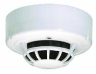
The 4351E thermal detector incorporates an Application Specific Integrated Circuit (ASIC). Combined with the latest in thermal element technology the detector provides efficient and accurate detection of fires, especially in environments such as boiler houses or kitchens where smoke detectors are inappropriate due to the high level of airborne contamination. The 4351E operates when the detected temperature exceeds 78°C.
