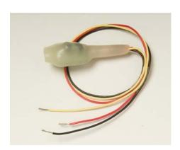
The VIGILANT PA0443 Contact Conversion Module is designed to allow normally-closed clean contact devices (e.g. manual callpoints) to be connected onto legacy (pre-NZS4512:2003) smoke detector circuits. The module converts the normally-closed hard contact to a normally-open transistor clamp (clamps to about 1 volt when the contacts open) across the detection circuit. For new (NZS4512:2010) installations, use PA1022.
