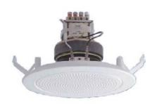
The 'One Shot' PA speaker and grille is designed to install easily into 10 to 13mm gyprock/plaster/ acoustic ceilings. Simply drill the required size hole, terminate the wiring and push the speaker into the ceiling until it snaps into place. They are designed to meet the requirements of AS2220.1, with a transformer cover and 22µF capacitor. The transformer has 5 power taps from 0.33 to 5W and a 4-way terminal block.
