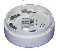
The 814RB Addressable Relay Base provides two sets of changeover volt-free relay contacts capable of switching 1A (resistive) @30Vdc. The relay function is controlled by the MX fire alarm panel via the detector fitted to the 814RB. The 814RB may be mounted directly to the ceiling or plugged into a 4B/5B, Universal or 4B-I/5B-I Isolator Base.
