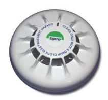
The 801PHEx Intrinsically Safe Optical Smoke & Heat Detector plugs into a 5BEx base. The detector is designed to transmit to a remote MX fire controller. digital signals which represent the status of the optical smoke and heat elements of the detector. Software within the controller interprets the returned optical and heat values to raise an alarm or other appropriate response according to the type of programmed configuration. The mode of detector
