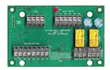
The MIO800 is a general purpose interface module for use with MX TECHNOLOGY fire detection systems. It allows multiple input and output connections to be made between external equipment and the MX DIGITAL loop. Three inputs and two relay outputs are provided. Each input on the MIO800 supports one of the following modes:
