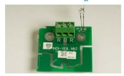
The Indi-VIGIL Indicating Module, when installed in a manual call point or wired to a cleancontact detector, is compatible with VIGILANT fire alarm systems in the same quantities as the indicating manual call point and Indi-VIGIL heat
