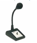
The SU0169 Desktop Paging microphone is a dynamic microphone with a cardioid polar pattern. It features a short-off press-to-talk (PTT) switch with an open-off type extra switch. It has low handling noise and a 600 ohm balanced output impedance. Compatible with the FP0539 Paging Console.
