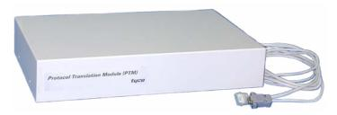
The Protocol Translation Module (PTM) provides an interface between VIGILANT fire panels on a Panel-Link network and a network event printer or an XL Graphics computer system. The PTM is programmable as to which panels/events are printed or sent to the XL Graphics system.
