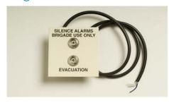
MEO433 consists of a set of (Trial) Evacuation and Silence Alarms 2-pole 2-way Bulgin keyswitches, pre-assembled and wired on a labelled White (Titania) plate. Both of these switches have their key removable in one position only to comply with NZS 4512:2003. The unit is designed to directly replace the MCP blanking plate in the standard 15U MX4428 configuration, but could also be used in other cabinet configurations, or be mounted directly to an index.
