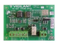
The ISO 8201 Strobe Driver generates an ISO 8201 compliant "T3" pattern for the Multi–Candela strobe 4906–9104. It connects directly to a supervised relay output of a fire alarm panel and drives one or more lines of strobes with a synchronised T3 pattern. The fire alarm panel's output supervision supervises the wiring from the panel to the strobes. The output signals of up to 5 modules can be synchronised. Four standoffs are supplied for mounting.
