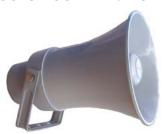
distributed paging systems where a high degree of speech articulation and program clarity is paramount. Typical applications include schools, train/bus stations, airports, car parks and plant rooms. An adjustable power tap switch is provided, as is a 22µF bipolar isolation capacitor to permit line monitoring function when employed with Warning System installations. A 4 core loop-through flying lead is provided.
