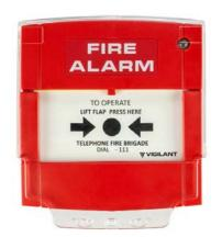
The VNCPI is a conventional indicating manual callpoint (MCP) that is suitable for indoor applications. It is supplied with a plastic element, which deforms when pressed in to release a microswitch.
