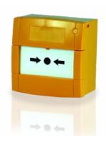
The FP1114 MCP is surface mounting, with a plastic coated glass element to ensure reliable, safe operation. It is coloured yellow (for use in gaseous suppression applications). The call point is operated when the glass element is snapped, releasing the MCP's micro switch. The element is snapped by pressing on its centre - a hammer, or other impact device, is not required.
