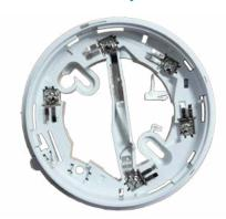
The 4B-C Continuity Base is used for most installations involving 850 Series detectors, as it allows the detector's in-built short circuit isolation function to be in-circuit when the detector is fitted and ensures continuity is maintained when the detector is removed. The 4B-C is not supported on MX4428.
