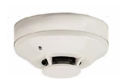
The P135A/2251TMB is a photoelectric smoke detector with supplementary 57°C thermal. The ACCLIMATE uses advanced on-board software to combine the signals from the photo and thermal elements. This software creates a true multicriteria detector capable of rejecting nuisance sources, but still responding quickly to real fires. It has the capability of adjusting its sensitivity according to the type of environment that it is installed in.
