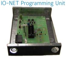
The IO-NET Programming Unit transfers the program to the IO-NET Controller PROMs. The Programming Unit is supplied complete with a cable to connect to a PC, the compiler programming software and the user manual. An external 24Vdc supply is required. IO-NET is also able to be programmed using SmartConfig Version 1.6 onwards. The IO-NET site specific configuration is stored in read-only memory. It may be re-programmed multiple times before requiring chip replacement
