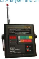
The STI-CIS Analyser measures the speech intelligibility of a fire alarm evacuation signal. To measure overall speech intelligibility, the STI-CIS Analyser uses the STI measurement method to factor in the effects of the warning system, room acoustics (reverberations and echoes) and background noise.
