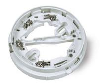
The 4B Universal Base contains no electronics and is suitable for indoor applications of the 614 series conventional (non-addressable), 814 and 850 series analogue addressable detectors. It provides excellent space for cable access and terminations. It features remote LED connections and an anti-tamper facility. The 4B base is designed to snap-fit into the ceiling tile adaptor, or screw fix to the ceiling in the traditional manner.
