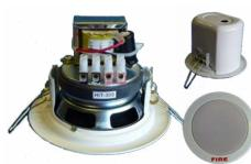
The SU0346 (HIT-300) is a 75mm fast-fit 100V Line Loudspeaker with a very low profile – only 70mm – which fits in most wall and ceiling cavities. It offers transformer-coupled 0.33W, 1.0W, and 2.5W power taps, plus an integral DC blocking capacitor. Spring-loaded clamps allow installation directly into an 86mm ceiling aperture without needing any other fixings. It offers clear sound reproduction of both emergency tones and voice messages.
