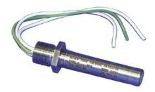
Constructed from stainless steel, the T54B is an extremely rugged heat detector that can be used to detect fires in the harshest of environments. The T54B can be used in environments with ambient temperatures up to 280°C and, being hermetically sealed, is impervious to most
