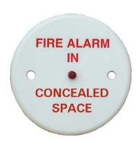
The E500 Mk2 range of remote indicators provide remote indication of an alarm condition on a fire detector. They are used where the fire detector is installed in an inaccessible location, and indication of alarm must be provided in an easily accessible area. For example, where the detectors are in roof spaces or cupboards, under the floor, or in hotel rooms, and indication is required in the room or corridor.
