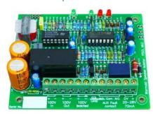
To prevent PA loudspeakers in a secure area from being used as microphones, the Speaker Isolation Module SIM-Mk2 is installed within the secure area between an incoming 100V speaker circuit and the speakers to be secured.
