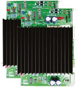
KT0519 200W Amplifier Module Kit The 200W amplifier comprises two PA0647 AMP200 PCB modules and one LM0141 FRC loom.
