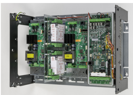
T-GEN 60 on FP1119 Bracket in PDI Expansion Bay with FP1118 Brackets & Splitter Modules
