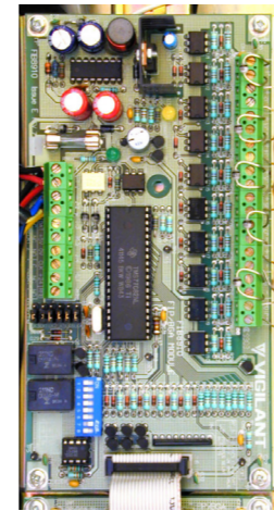
FP1068 FIB8910 (PA0651) FIP/BGA Master Module DD0084 FIP EOL Zener Diode
