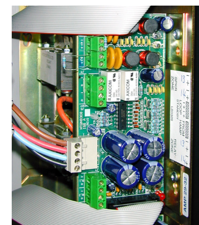
PA0691 HTRN9308-1 2x50W Transformer Module PA0695 HTMS9408-2 2x50W Transformer Music Switching Module
