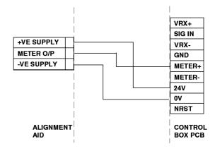
Fig. 3 Connection of Alignment Aid
