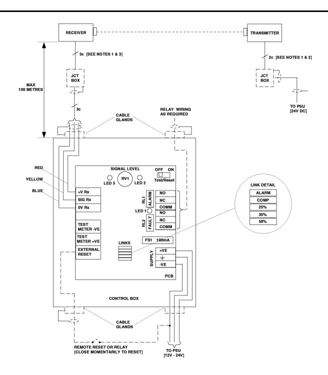
NOTE 1: BOTH THE TRANSMITTER [TX] AND RECEIVER [RX] UNIT ARE SUPPLIED WITH 1 METRE [NOMINAL] OF FACTORY CONNECTED 4-CORE CABLE [UNSCREENED].
