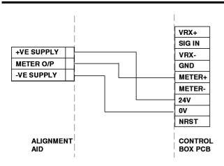
Fig. 3 Connection of Alignment Aid
