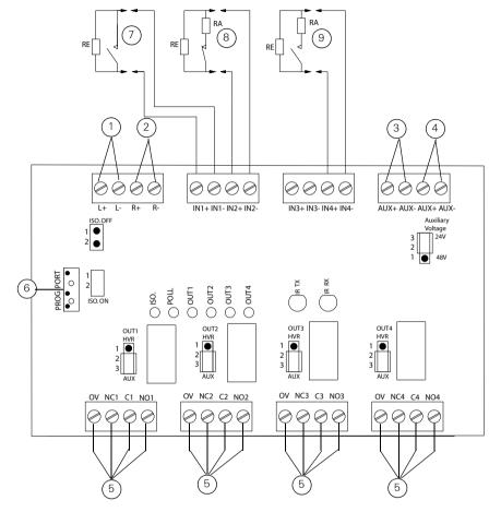
Fig. 3: Terminal Arrangement
