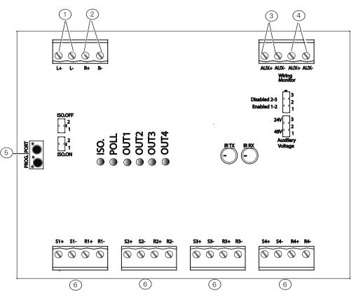
Fig. 3: Terminal Arrangement
