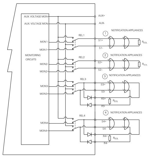
Fig. 4: Monitored Spur and Loop Relay Configuration
