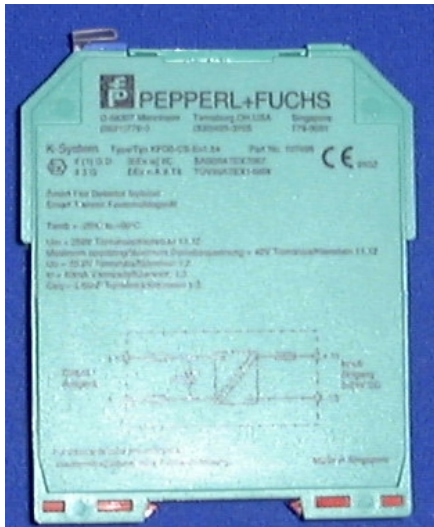
Fig. 1 Pepperl + Fuchs KFD0-CS-Ex1.54 Galvanic Isolator
