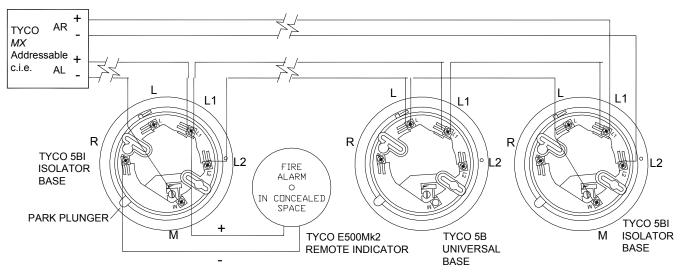
The MX c.i.e. can be programmed to illuminate a Remote Indicator for detectors in alarm other than the detector base to which the Indicator is connected.
