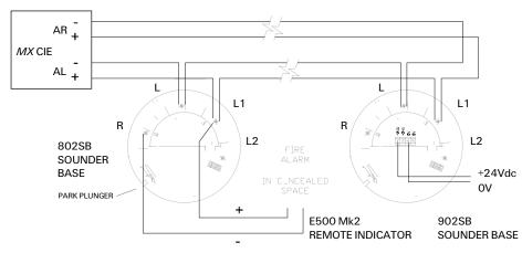
Note: The *MX* CIE can be programmed to illuminate a Remote Indicator for detectors in alarm other than the detector base to which the Indicator is connected.
