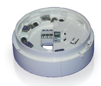
The 814RB MX Addressable Relay Base provides two sets of change-over volt-free relay contacts capable of switching 1A (resistive) @30Vdc. The relay function is controlled by the VIGILANT MX Control and Indicating Equipment (CIE) via the addressable detector fitted to the 814RB. The 814RB may be mounted to the ceiling, or plugged into a 4B Universal base or 4B-I Isolator base or 4B-C Continuity base.
