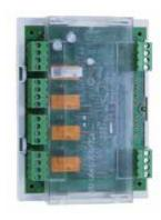
The Quad Relay Output module provides four voltage-free change-over relay outputs or switched auxiliary supply (24V/48V selectable) outputs. Supervision of the auxiliary supply can be enabled to detect disconnection or failure. The QRM850 includes an *MX* loop short-circuit isolator and can be programmed using the IR link from the 850EMT.
