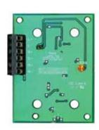
The LIM800 Loop Isolator Module can be used to provide short circuit isolation between zones or portions of an MX addressable loop. LIM800s are installed at appropriate positions around the MX loop to monitor the loop voltage either side of the device. If a short circuit is detected, the two LIM800s either side of the short isolate the shorted section allowing the rest of the loop to be driven by the CIE.
