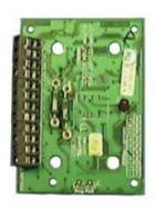
The DIM800 Detector Input Module interfaces two conventional detector circuits onto the *MX* addressable loop. Each circuit can support 3mA of detector quiescent current and requires a 4k7 Ohm End Of Line resistor. Unused circuits must be terminated with an ELD resistor. The DIM800 requires a suitably rated and separately protected external 24V supply to power the detector circuits. The two circuits are available as separate subpoints and can be mapped to different zones on the CIE.
