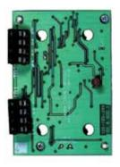
The CIM800 Addressable Contact Input Module supervises 2 circuits of voltage-free contacts. The CIM800 can be configured to monitor:
