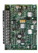
The DDM800 Universal Fire & Gas Detector Module is designed to monitor and signal two conventional 2-wire 20V fire detector circuits (or two 4-20mA current loop sensors on MX4428).
