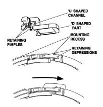
Fig. 5 Fitting Address Label Carrier
