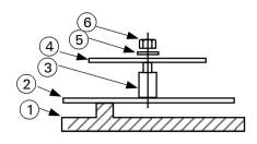
Fig. 3: ANC-8 - PCB Fixing Detail
