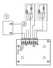
Fig. 8: Spur Circuits (Class B) Normally Open Contacts Short Circuit A+ to A- or B+ to B-= Fault
