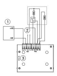
Fig. 10: Loop Circuit (Class A) Normally Open Contact Short Circuit A+ to A- or B+ to B-= Fault
