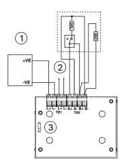
Fig. 9: Loop Circuit (Class A) Normally Closed Contact Short Circuit A+ to A- or B+ to B-= Fault
