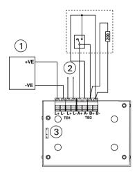
Fig. 12: Loop Circuit (Class A) Normally Open Contacts Short Circuit between A+ and A- or B+ and B- = Alarm
