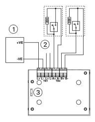
Fig. 11: Spur Circuit (Class B) Normally Open Contacts Short Circuit between A+ and A- or B+ and B-= Alarm
