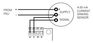
Fig. 13: Connection of a 4-20 mA current sinking sensor (only one circuit shown for clarity)
