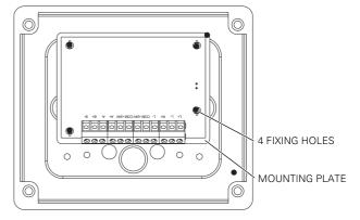
Fig. 5: DDM800 in the D800 housing
