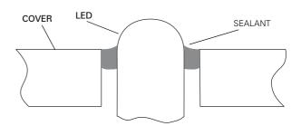
Fig. 7: Sealed LED
