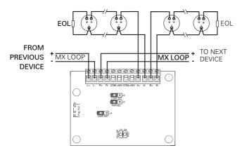
Fig. 9: Spur circuits loop powered
