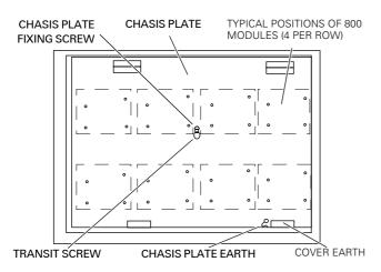
Fig. 3: ANC8 - Chassis plate
