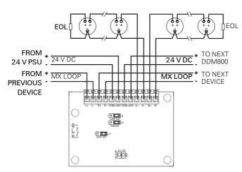
Fig. 8: Spur circuits with external 24 V
