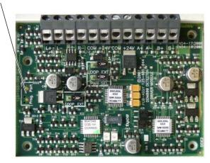
Fig. 1: DDM800 - Universal fire and gas detector module
