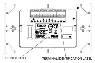
Fig. 4: DDM800 - Label positioning
