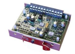
Fig. 6: DDM800 on DIN rail mounting bracket
