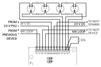
Fig. 10: Loop circuits (Class A wiring) with external 24 V
