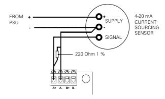
Fig. 14: Connection of a 4-20 mA current sourcing sensor (only one circuit shown for clarity)
