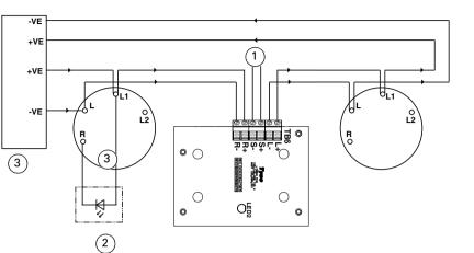
Fig. 6: LIM800 Line Isolator Module - Simplified Wiring Diagram
