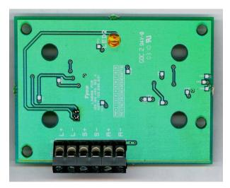
Fig. 1: LIM800 Line Isolator Module
