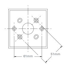
The MCP820 may be fitted to a standard (surface mounting) call point back box which is available separately.
