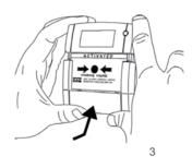
A test key is provided with each MCP to allow easy testing of the switch mechanism and wiring, without breaking the frangible element. The key is inserted into a slot in the base of the MCP, allowing the frangible element to drop away from the switch, thus activating it and registering an alarm at the CIE. Note: the key should not be left with the MCP after commissioning, but may be left inside the CIE for convenience.
