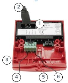
The MCP820 has a factory set (invalid) address of 255. The MCP820 is field programmed with the address prior to installation using an *MX* address programming tool. The associated ancillary programming lead plugs into the programming port.
