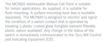
The MCP820 has an integral short-circuit isolator for monitoring the addressable loop wiring. The integral LED indicator is normally off. When the frangible element is broken, an alarm is registered and the LED will illuminate red. If a section of the loop wiring adjacent to the MCP820 is shorted, the built-in shortcircuit isolator trips, isolating the shorted section and the LED is illuminated yellow. The status remains until the short is removed.
