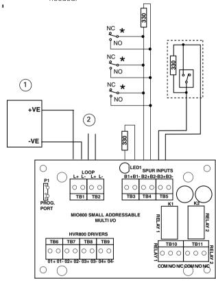
Fig. 7: Spur Circuit (Class B) Normally Open Contacts Short Circuit = Alarm
