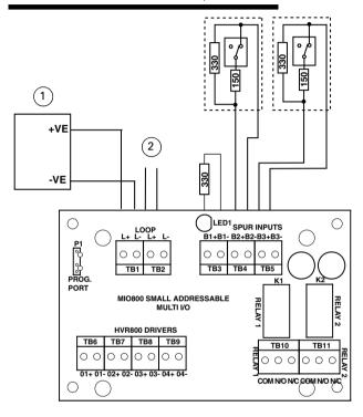
Fig. 6: Spur Circuits (Class B) Normally Open Contacts Short Circuit = Fault
