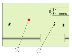
Fig. 2: RIM800 Relay Input Module Facia Plate 1– Address setting port 2– LED
