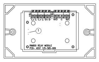
Fig. 3: RIM800 Simplified Wiring Diagram 1– Address setting port
