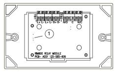
Fig. 6: RIM800 Fitted to Cover 1– Address programming port
