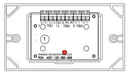
Fig. 8: SNM800 Fitted to Cover 1 - Address programming port
