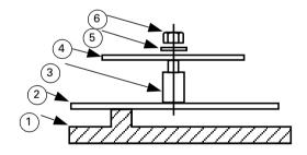
Fig. 7: ANC-8 - PCB Fixing Detail
