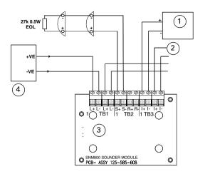
Fig. 3: Simplified Wiring Diagram showing Sounders wired in a Spur Configuration
