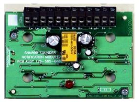
Fig. 1: SNM800 Sounder Notification Module
