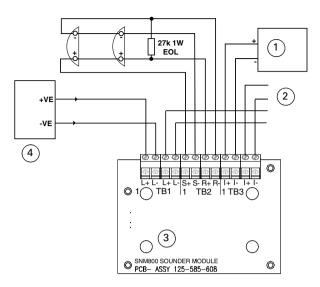
Fig. 4: Simplified Wiring Diagram showing Sounders wired in a Loop Configuration Note: The EOL must be physically mounted to terminals R+ and R-
