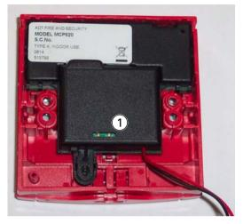
Fig. 3: CP820/CP820M - Address Programming Ports 1–Address programming port
