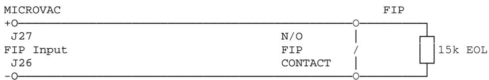
Short Circuit Fault Monitoring not used. (Switch 2:2 ON)
