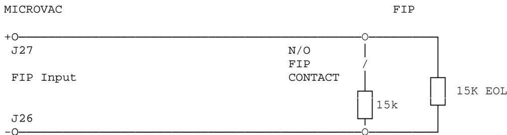
Short Circuit Fault Monitoring used. (Switch 2:2 OFF)
