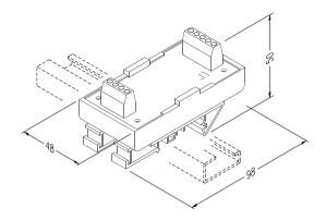
Figure 6 - Layout and dimensions with plastic DIN rail mounts (supplied)
