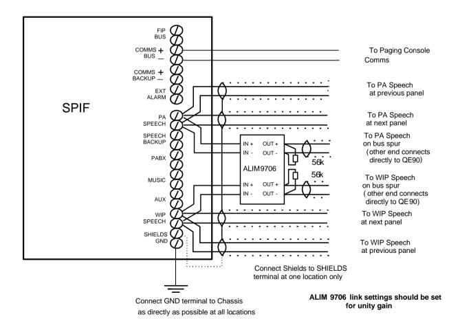
Figure 5 - Use of ALIM9706 at QE90 Network Spur
