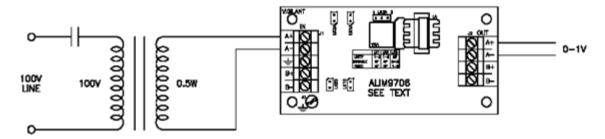
The links on the ALIM9706 should be: LK1 and LK2 not fitted, LK3 in position 2-3 to provide volume control.
