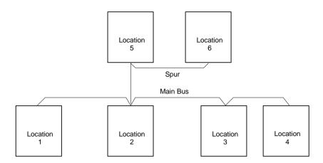
Figure 4 - Typical QE90 Network System (with spur)
