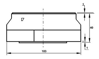
Fig. 1 Detector Base and Skirt Overall Dimensions
