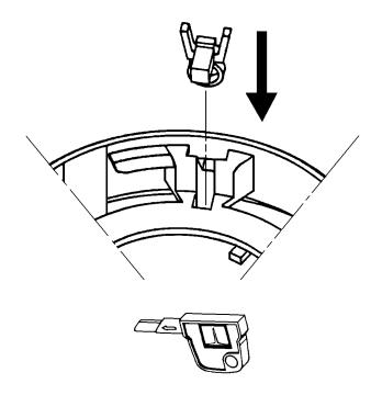
Fig. 4 Lock Insertion and key
