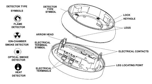
Fig. 2 Detector Base and Skirt
