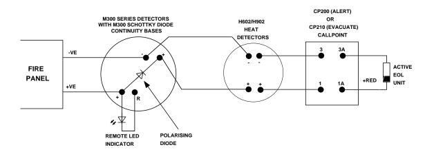
Fig. 9 Simplified Wiring Diagrams
