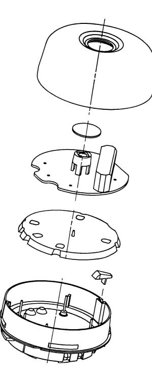
Fig. 3 General Assembly, Type MS302Ex Flame Detector
