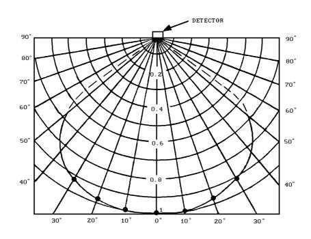
Fig. 7 Relative Range vs Angle of Incidence
