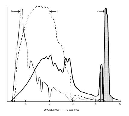
Fig. 1 Spectrums of a) Typical Carbonaceous Fire b) Solar Radiation at ground level c) Tungsten Filament Lamp
