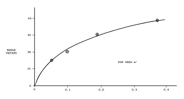
Fig. 6 Typical Detection Range vs Pan Area - Petrol
