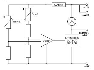
Fig. 1 Simplified Block Schematic Diagram
