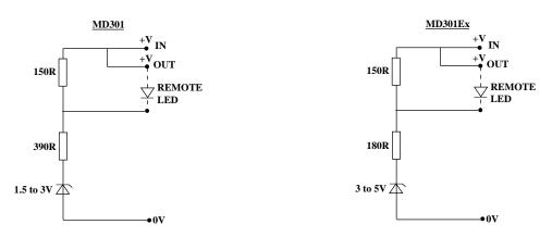
Fig. 4 Alarm Load Presented to the Controller by the Detector
