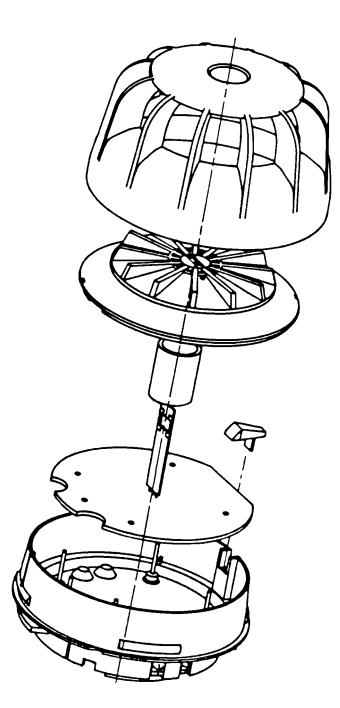
Fig. 2 General Assembly, MD300 Heat Detector
