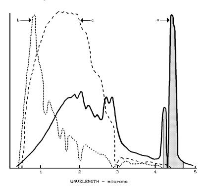
Fig. 1 Spectrums of a) Typical Carbonaceous Fire b) Solar Radiation at Ground Level c) Tungsten Filament Lamp 01A-04-D4 03 2/97
