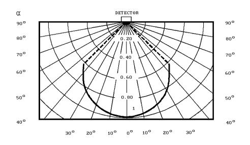
Fig. 5 Relative Range vs Angle of Incidence
