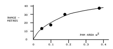
Fig. 4 Detector Range vs Pan Area - Petrol
