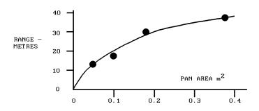
Fig. 8 Detection Range vs Pan Area - Petrol
