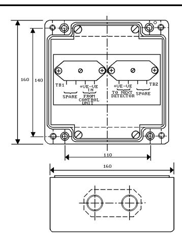
Fig. 3 S161 Housing showing Fixing Dimensions
