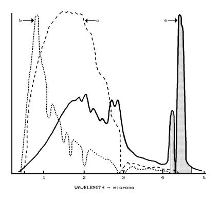
Fig. 1 Spectrums of a) Typical Carbonaceous Fire b) Solar Radiation at Ground Level c) Tungsten Filament Lamp The hazardous area classification, together with the mechanical design, allows the detector to be used as a direct replacement for flameproof detectors such as the DETECTOR ELECTRONICS U7600 and U7698.
