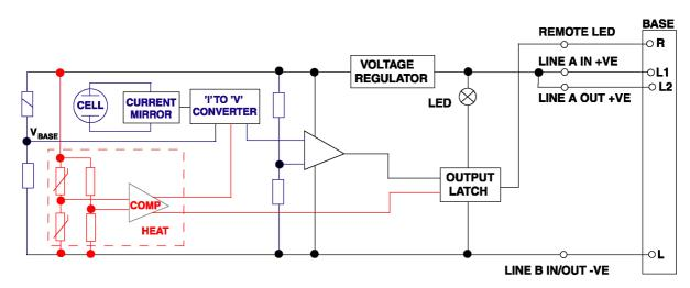
Fig. 2 Simplified Block Schematic Diagram of Detector
