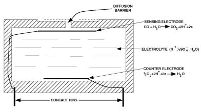
Fig. 1 Representational Diagram of CO Sensing Cell
