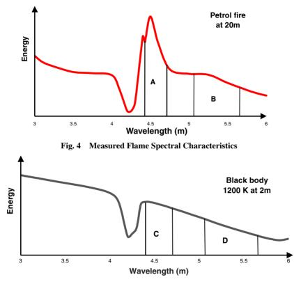
Fig. 5 Measured Blackbody Spectral Characteristics
