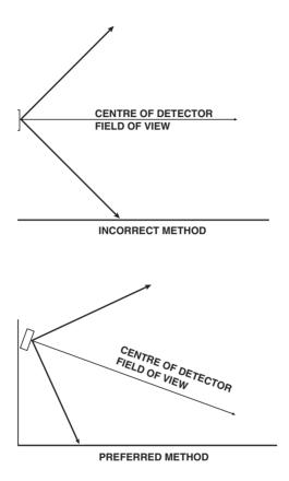
Fig. 24 Detector Orientation Relative to Horizon
