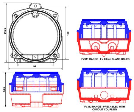
Fig. 11 FV300 Series - Overall Dimensions
