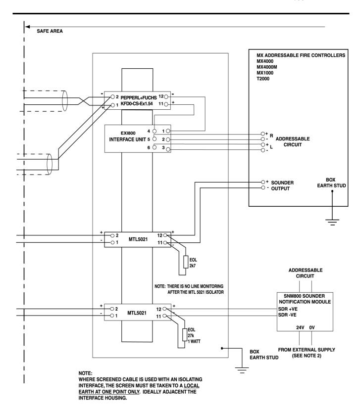
Fig. 5b) I.S. Interconnection Diagram to MX Addressable Fire Detection Systems
