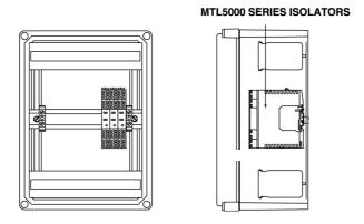
Fig. 4 DX170 Overall Dimensions Showing Mounted MTL5000 modules
