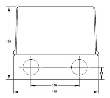
Fig. 1 Overall and Fixing Dimensions for UC2 4-Way Housing - for I.S. Sounder Driver/EXI800 MX Loop Interface/Galvanic Isolator
