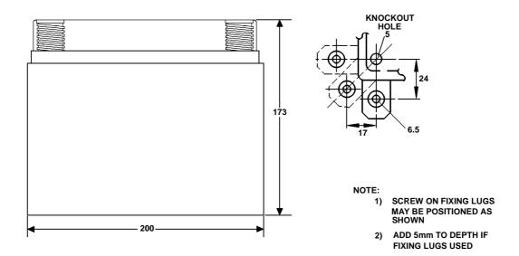
Fig. 2 Overall and Fixing Dimensions for UC4 8-Way Housing- for I.S.Sounder Driver/EXI800 MX Loop Interface/ Galvanic Isolator
