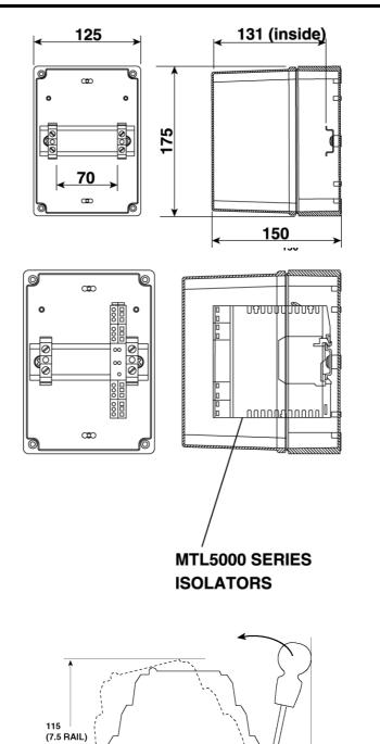
CLEARANCES (MM) FOR FITTING AND REMOVING BARRIERS
