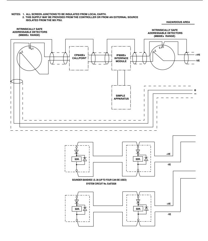
Fig. 5a) I.S. Interconnection Diagram to MX Addressable Fire Detection Systems
