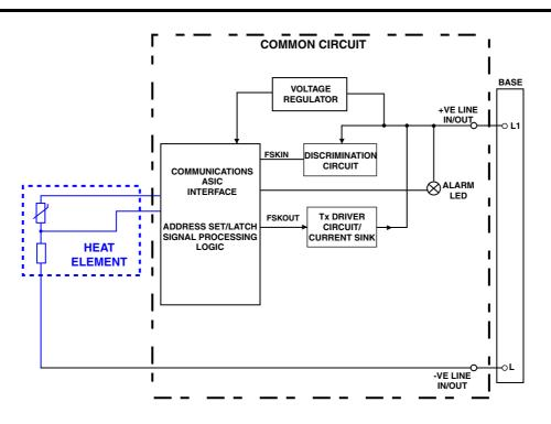
Fig. 1 Simplified Block Schematic Diagram
