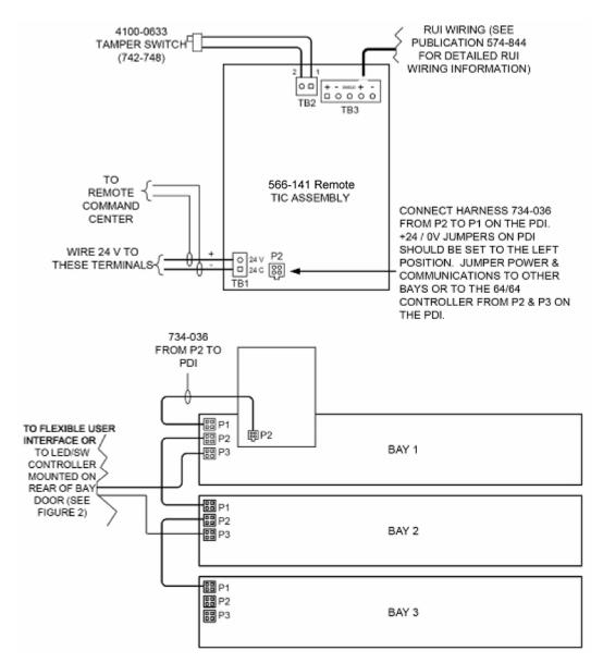
Figure 3. Wiring for 4100-9611, 4100-9612, 4100-9613, and 4100-9614. TIC Assembly Used on the the Remote Annunciator
