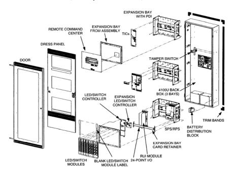
Figure 1. 4100-9607, -9608, -9609, & -9610 Remote Annunciator Installation (4100-9610 Shown)
