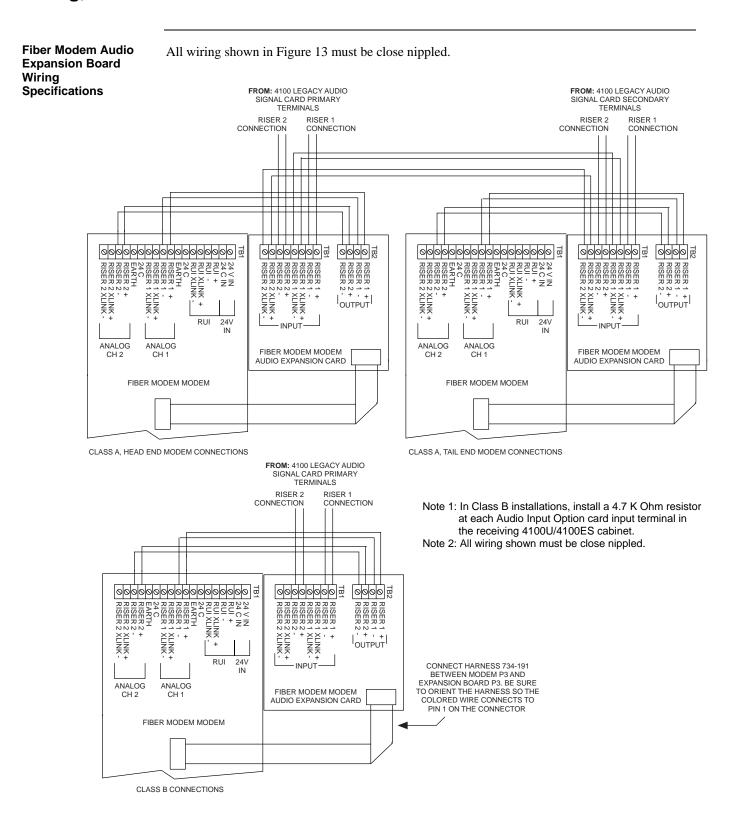
Figure 13. Modem Audio Expansion Board Wiring Diagram
