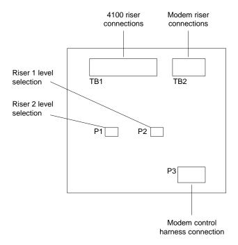
Figure 2. Fiber Modem Audio Expansion Board
