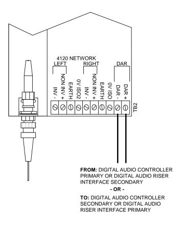
Figure 11. Modem to Digital Audio Riser Wiring Diagram
