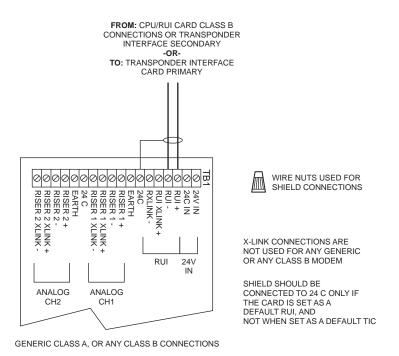
Figure 12. Modem to RUI Wiring Diagram
