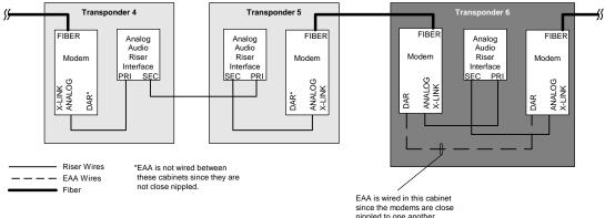
Figure 10. Enhanced Analog Audio Combinational System Wiring Diagram
