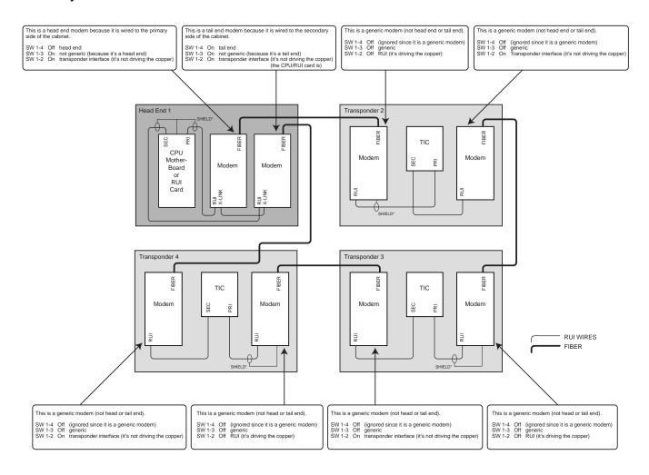
Switch 1-5 (Enable RUI interface) and Switch 1-1 (Class A wiring) both ON for all modems in this configuration.
