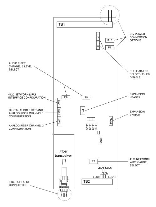
Figure 1. Fiber Optic Modem Board
