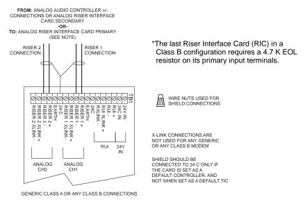
Figure 8. Modem to Analog Audio Riser Wiring Diagram
