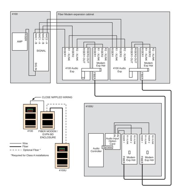
Figure A-21. Fiber Modem Audio Expansion Board, Class A/Style 6 (4100U Shown)
