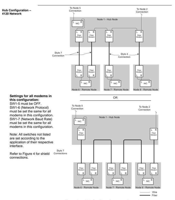
Figure A-13. Hub Configuration – 4120 Network
