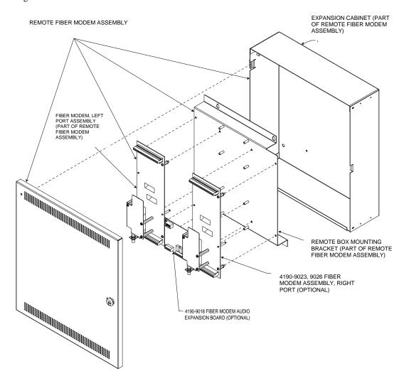
Figure 4. Modem and Audio Expansion Board Mounting in a 4190 Remote Expansion Cabinet
