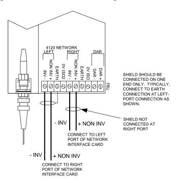
Figure 7. Modem to 4120 Network Wiring Diagram
