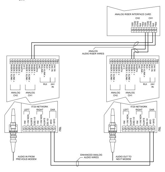
Figure 9. Modem to Enhanced Analog Audio Riser Wiring Diagram
