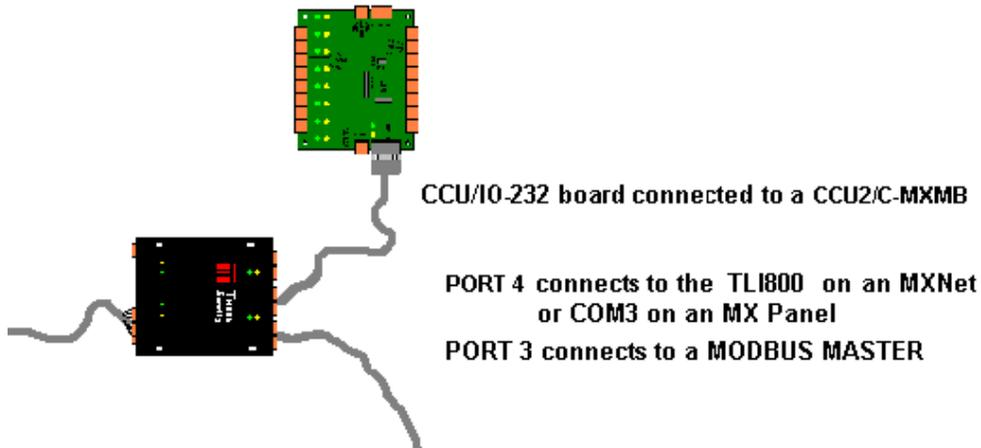
**Figure 10: Connection of a CCU/IO-232 or CCU/I-232 to a CCU2/C-MXMB**
