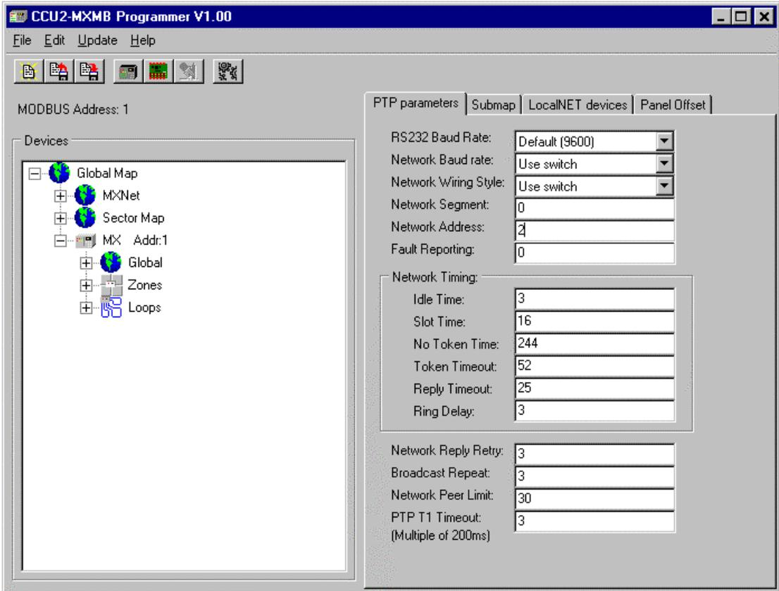
Figure 20: Setting PTP Parameters
