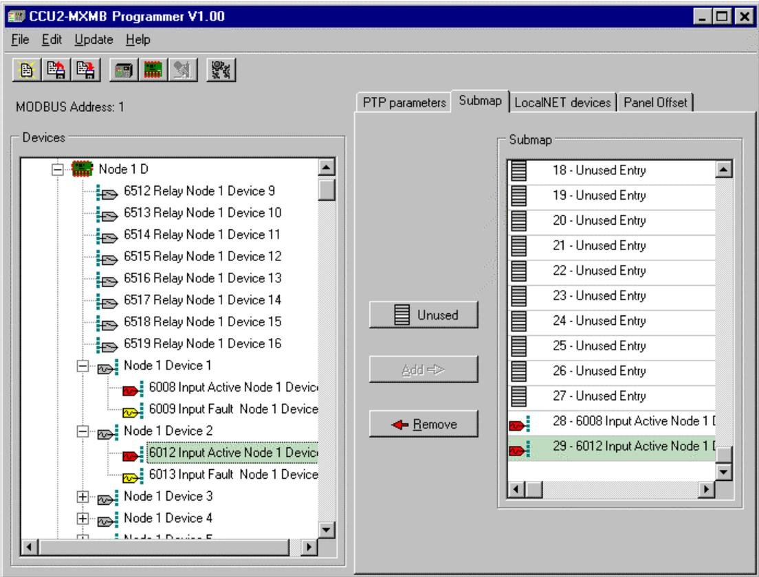
Figure 26: Adding the Input Active bits to the submap
