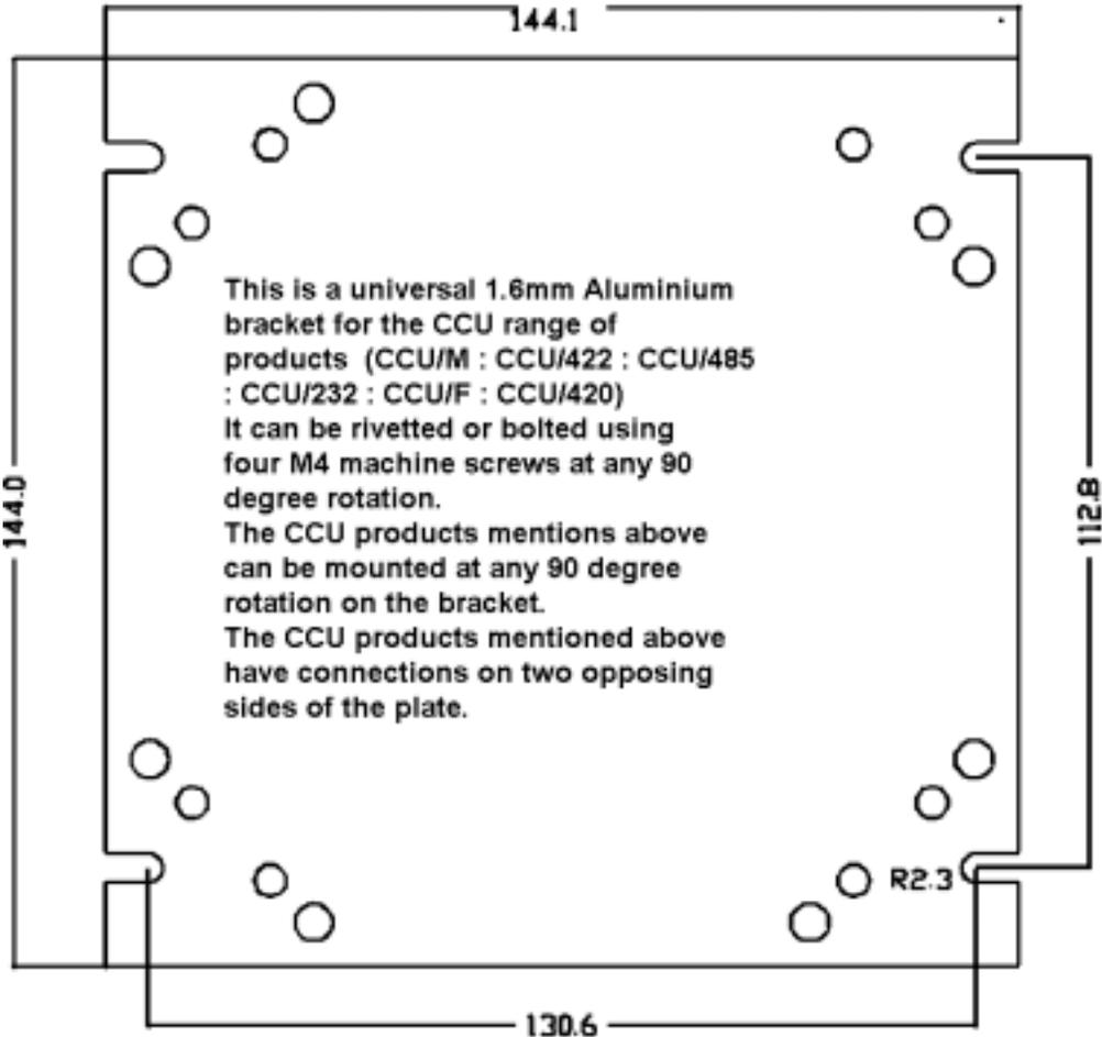
**Figure 3: Mounting Bracket**
