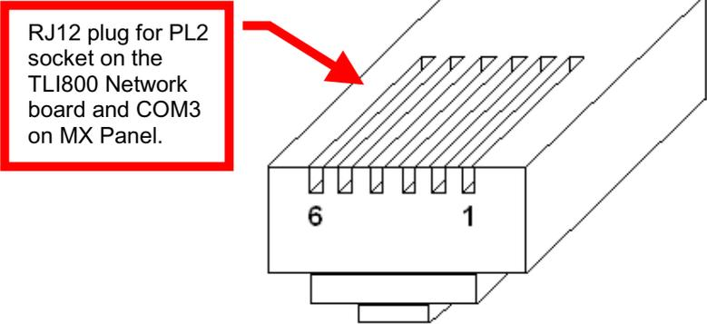
Figure 5: RJ12 Plug for TLI800 and COM3 Panel Connection.
