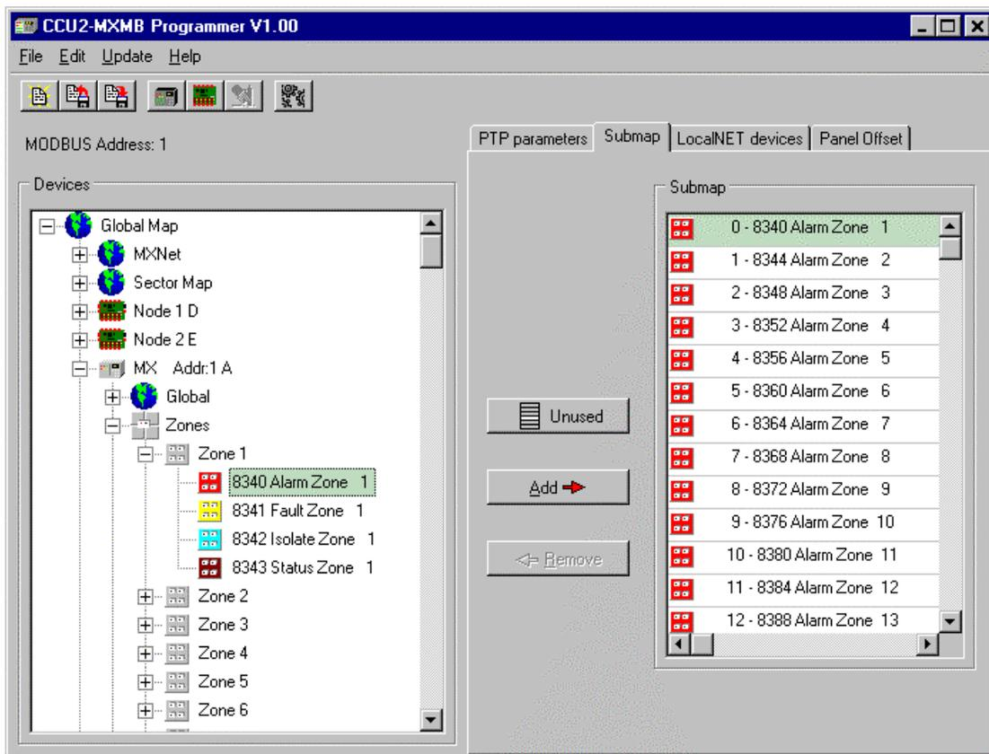
Figure 25: Adding the Zone Alarm bits to the submap
