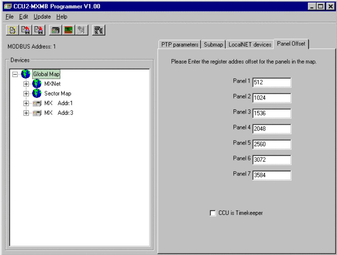
Figure 21: Setting Panel address offsets Parameters
