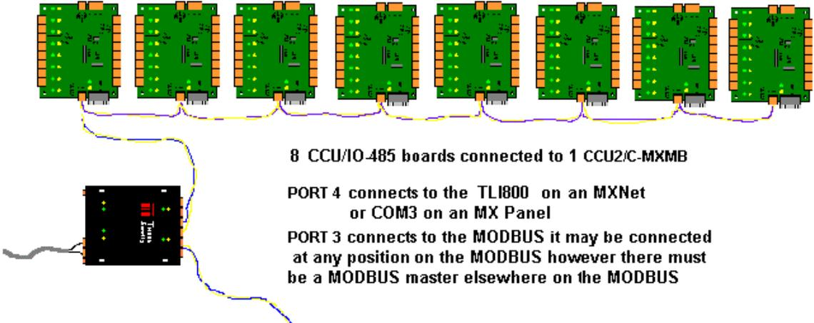
**Figure 9: Connection of CCU/IO-485(s) to a CCU2/C-MXMB**
