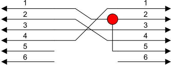
RJ12 TLI800 Connector                      Port 4 CCU2/C-MXMB
