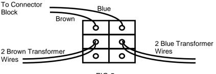
FIG 5 REAR VIEW OF SWITCH IN CORRECT ORIENTATION
