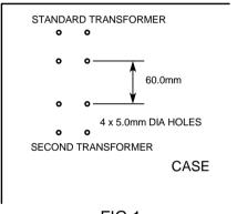
FIG 1 TRANSFORMER MOUNTING - DRILL DETAIL
