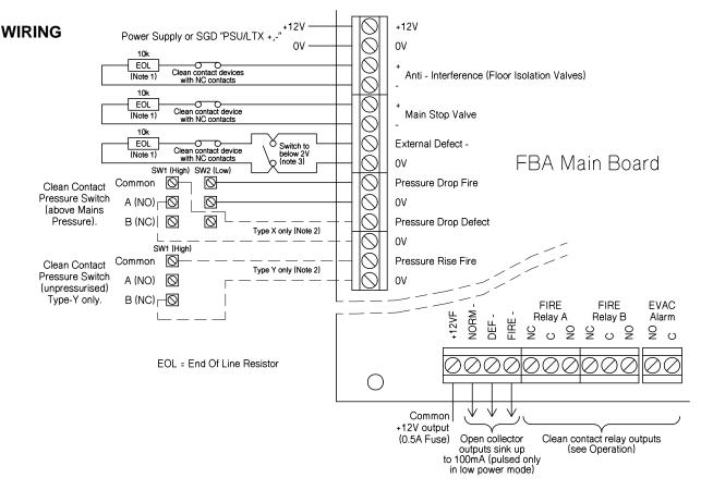
Note 1: If any of the Anti-Interference, Main Stop Valve, or Ext Defect- inputs are not used the 10k EOLR must be fitted to normalize the input.
