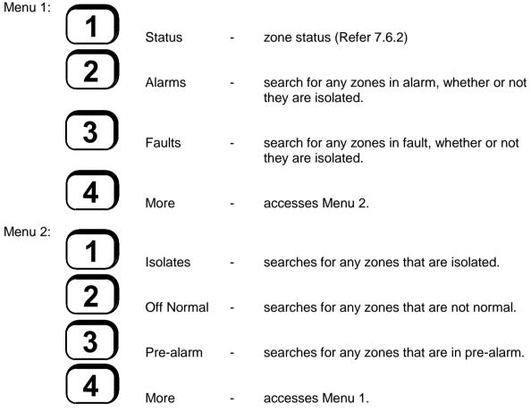
The MX4428 searches itself for a zone that meets the specified criteria from ACZ 0 up to the programmed maximum LCD zone. If none is found the MX4428 then polls the other FIPs on the network to determine whether they have any zones that meet the criteria.
