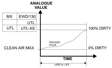
The % Dirty level of a detector is then determined by calculating how far between Clean Air Max and UTL(MX) or UTL-AS (EWD/130 series) the TV is.
