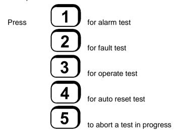
The MX4428 will then send the test command to the FIP with the selected zone on it.
