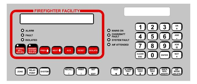
FIGURE 2.2 MX4428 AS4428.1 FIP KEYPAD LAYOUT
