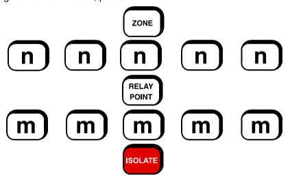
The LCD will display the selected range of zones, i.e. zone nnnnn to zone mmmmm inclusive, plus the options to isolate or de-isolate the range.
