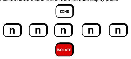
The LCD will display the selected network zone, and the current isolate status of the zone is retrieved from across the network. There may be a delay of a few seconds before this is displayed. Wait until the data is displayed before proceeding.
