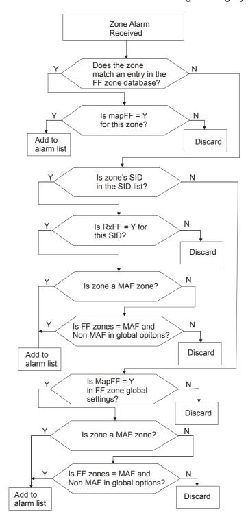
FIGURE 3.4.1 Processing of Network Alarm Messages
