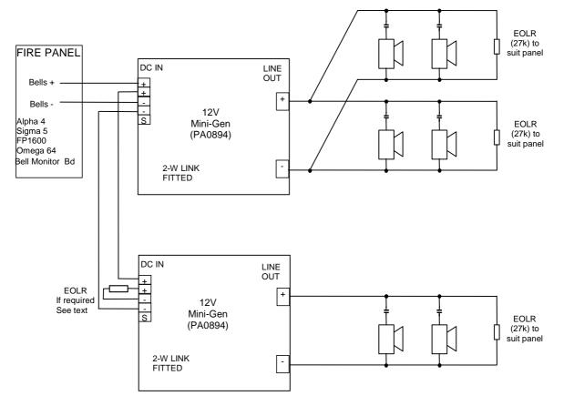
Fig 1 Example of Multiple Branches on Fire Panel with Bell 3 Branch Supervision
