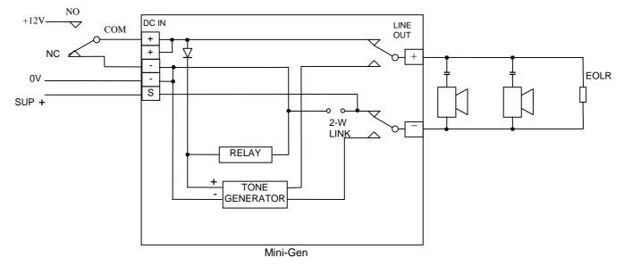
Fig 2 Mini-Gen Connection With Separate Supervision (single pole / 4 wire)
