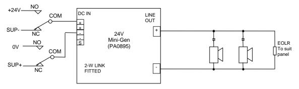
Fig 3 Mini-Gen Connection For Two Pole Relay With Integral Supervision (2 pole / 2 wire)
