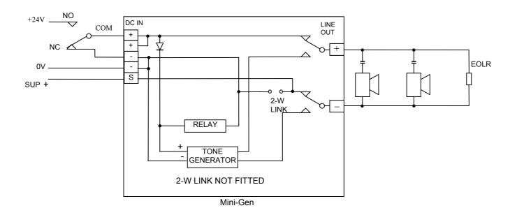
Fig 2 Mini-Gen Connection With Separate Supervision (single pole / 4 wire)
