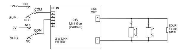
Fig 3 Mini-Gen Connection For Two Pole With Integral Supervision (2 pole / 2 wire)
