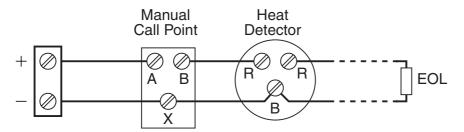
Thermal / Combined Circuit Wiring
