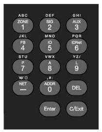
Figure 5-1. Function/Numeric Keypad
