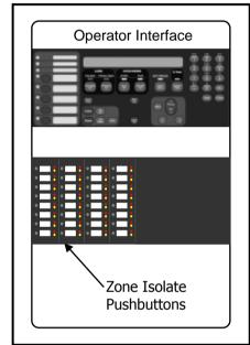
The panel is reset by pressing <SYSTEM RESET>. If the alarm won't reset the point may still be activated. Press <FIRE ALARM ACK> when the point alarm is displayed, then press <DISABLE>, <ENTER>. Press <FAULT ACK> (to acknowledge the fault caused by disabling a point), then press <SYSTEM RESET> again. The disabled detector must be re-enabled when the condition is cleared.
